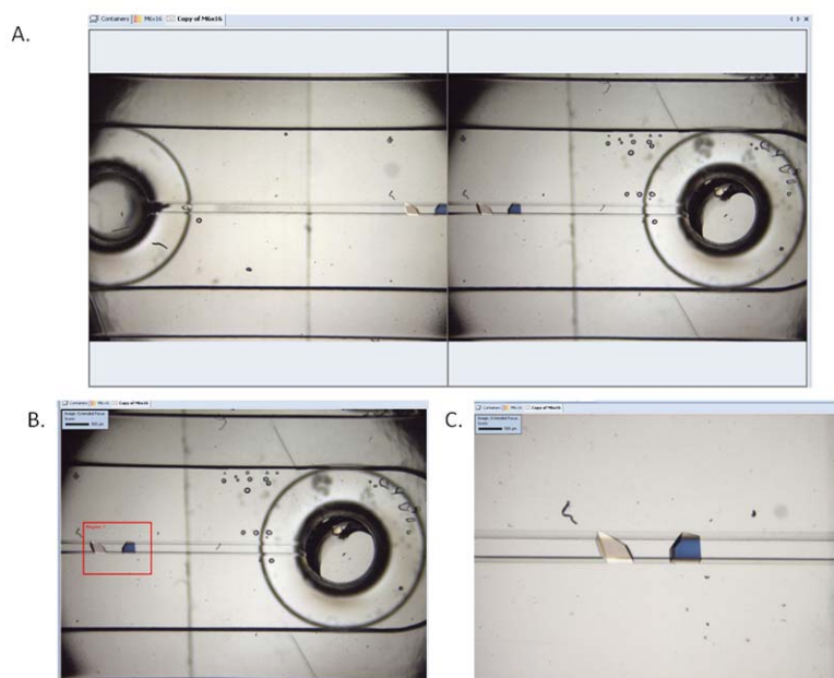
Figure 3 | Imaging of the 96-channel Crystal Former with the Rock Imager. (A) An overview of the user interface with the 96-channel Crystal Former defined. (B) A magnified overview of the user interface. (C-D) Individual “drop” images, each comprise one-half of a single microchannel. (E) The whole channel view for a single microchannel in the 96-channel Crystal Former.
